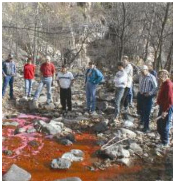
Figure 8. Stream injected with Rhodamine dye at Custer Gap disappears a short distance downstream on Boxelder Creek (photo courtesy of Derric Iles, South Dakota Geological Survey).
