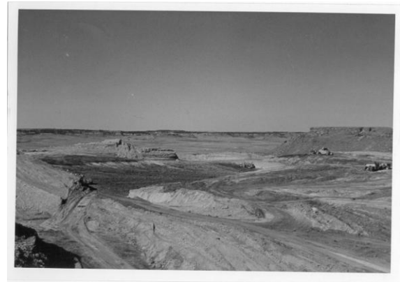
Figure 12. Uranium mining in the Riley Pass district ca. early 1960s. Overburden was pushed over the side of the butte to expose the uranium-bearing lignite units. USFS image.
