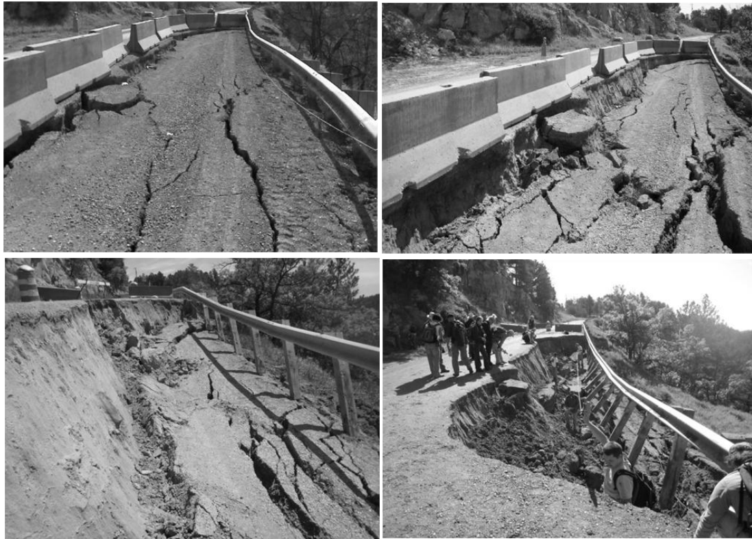
Figure 15. (a) The Sly Hill Road failure on May 11, 2009 (Photo Courtesy of the City of Sturgis, SD). (b) The Sly Hill Road failure on May 18, 2009 (Photo courtesy of the City of Sturgis, SD). (c) The Sly Hill Road failure on May 31, 2009. (d) The Sly Hill Road failure with students obtaining measurements on June 8, 2009.
