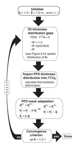
Fig. 8. Adaptive mesh algorithm.
