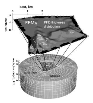
Fig. 5. FEM configuration. The tessellation consists of 12,400 elements and 14,574 nodes. The bottom portion of the figure represents the problem domain, which includes a PFD embedded in the substrate. The shaded relief image in the upper portion of the figure shows an expanded view of the PFD thickness distribution for FEM<sub>A</sub>. The thickness contour interval is 20 m. Circles outlining the PFD thickness distribution are nodal positions that outline the assumed lateral extent of the PFD.
