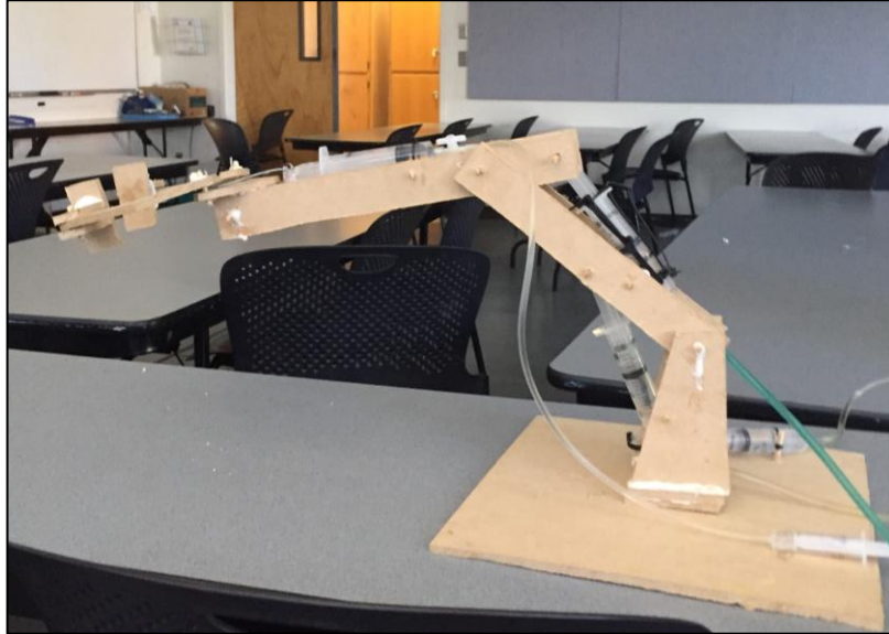
Figure 3. Side view of finished hydraulic claw.
