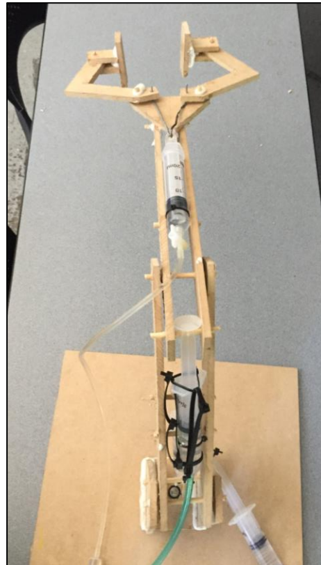
Figure 4. Top view of finished hydraulic claw
