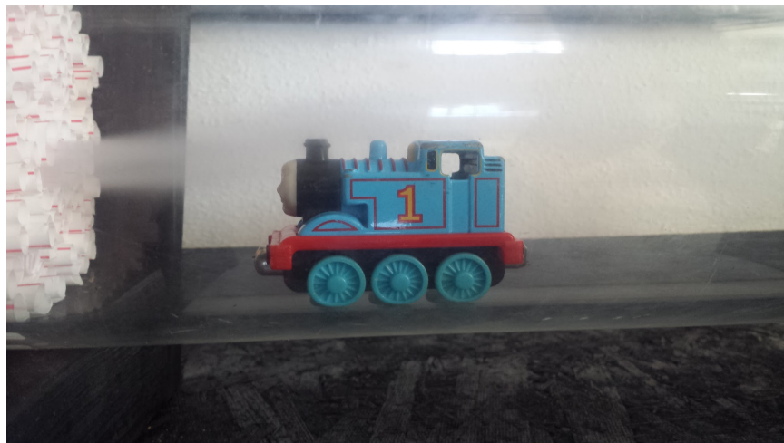
Figure 4: Testing of the model train. Notice the steady stream (left) breaking up over the top
